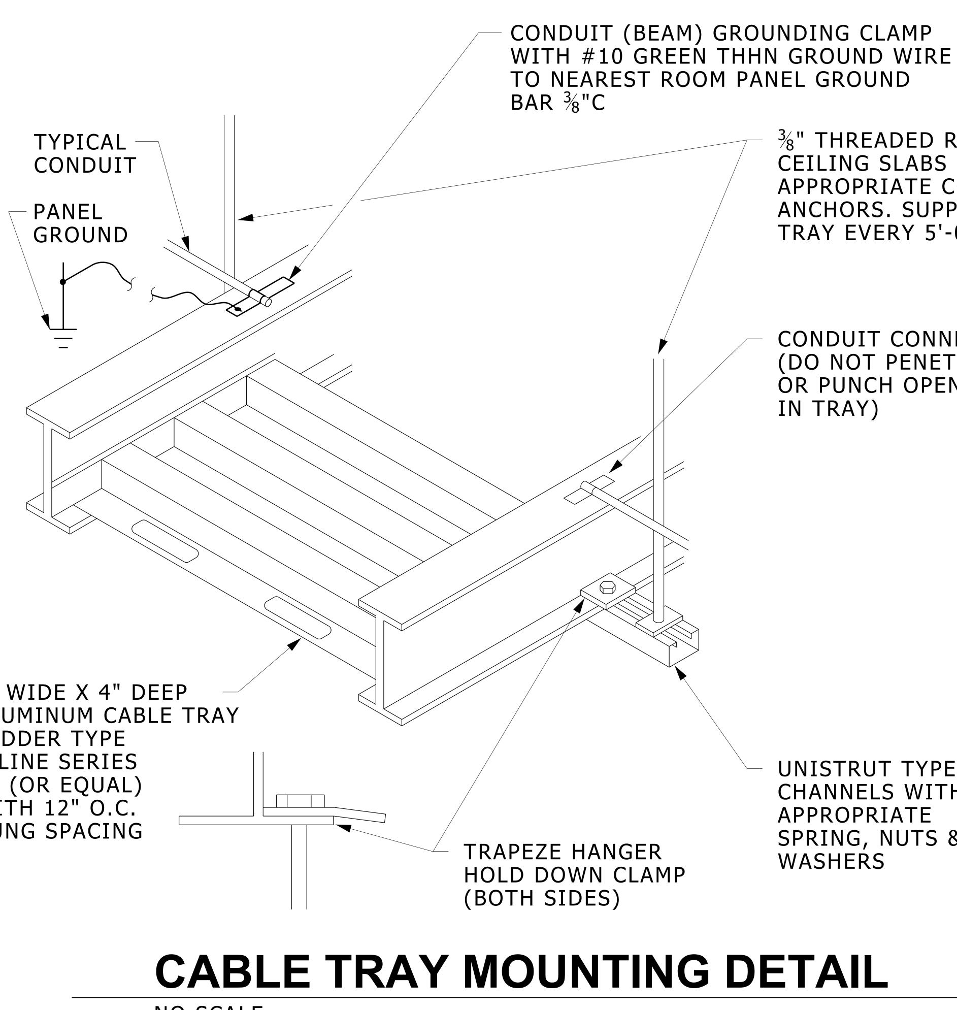
6" WIDE X 4" DEEP ALUMINUM CABLE TRAY LADDER TYPE **B-LINE SERIES** 24 (OR EQUAL) WITH 12" O.C. RUNG SPACING
